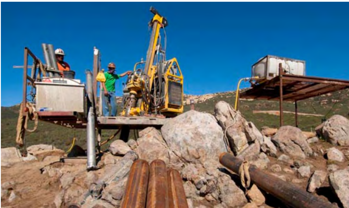
Photograph 2. Platform drill rig similar to what may be used to drill LT-B4.
