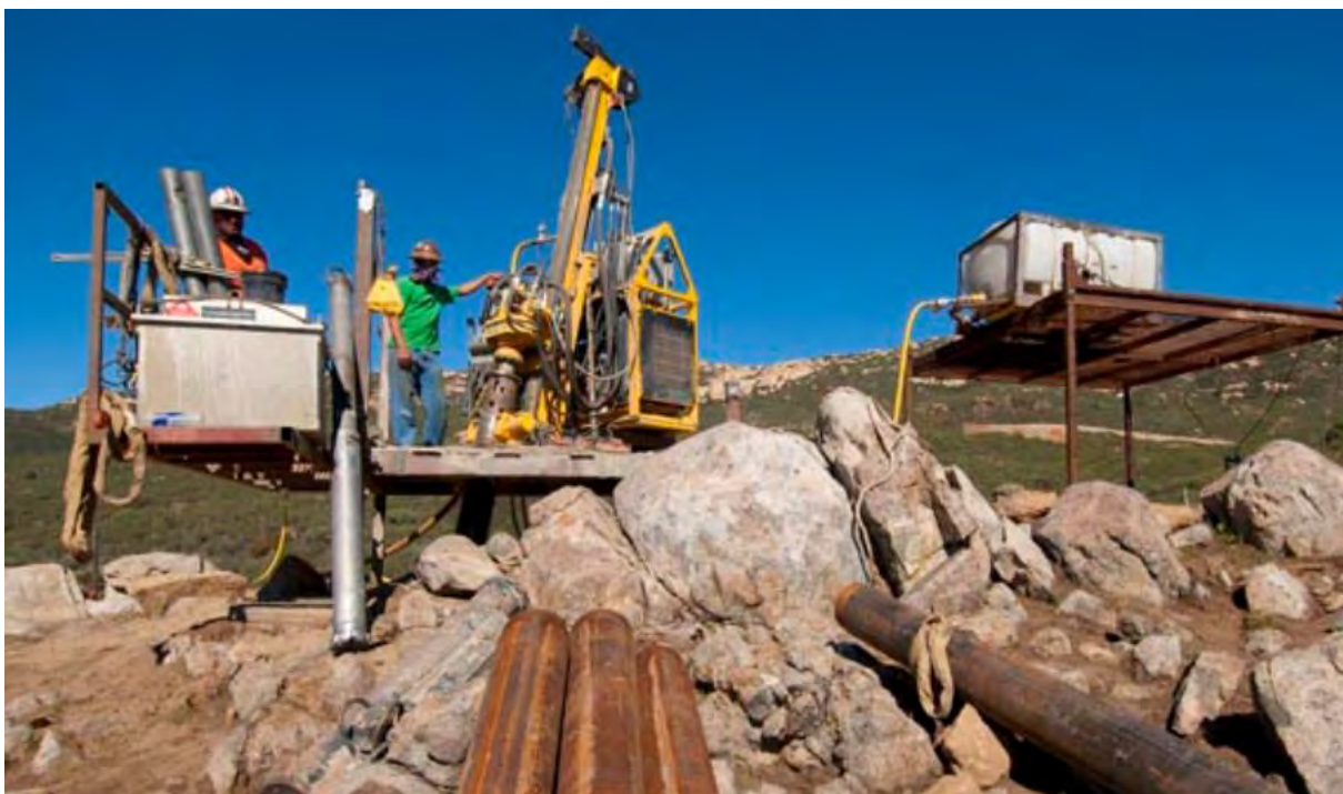
Photograph 2. Platform drill rig similar to what may be used to drill LT-B4.
