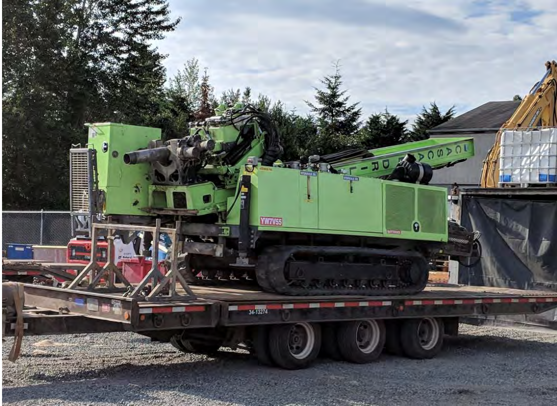
Photograph 3. Tracked drill rig similar to what may be used to drill borings other than LT-B4.
