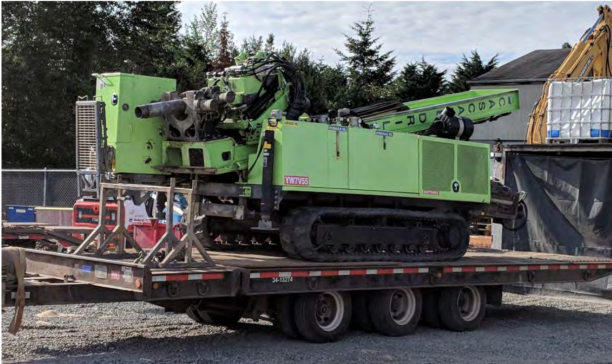
Photograph 1. Tracked drill rig similar to what may be used to drill borings other than LT-B4.
