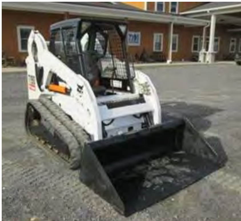
Photograph 6. Typical skid-steer, similar to what would be used to support drilling activities.
