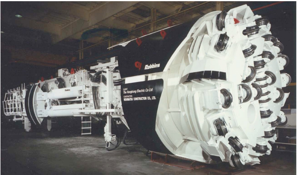
Figure 4-10. Main Beam Gripper TBM with Trailing Gear
